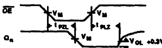
Waveform 5. 3-State Output Enable Time To Low Level And Output Disable Time From Low Level
